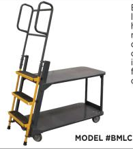
Ballymore introduces the heavy duty merchandise ladder cart with a capacity of 1,000 lbs. The cart has two large shelves for transporting a variety of merchandise. Ladder portion has a spring loaded device which secures the ladder to the floor when climbing and retracts for easy maneuvering. Cart is equipped with 4 casters- 2 swivels and 2 rigid for effortless turning and moving. Durable powder coated gray with yellow steps.
