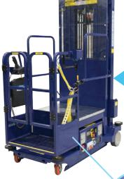
Power Stocker's optional sensing system creates a safety zone perimeter around the lift when in the raised position.
